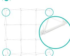
• Connect the top and bottom End Caps on each side of the frame.
