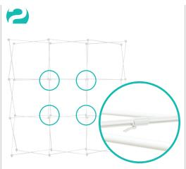
Close frame by pushing the outside of the frame until male and female ends connect. Repeat for all connectors.
