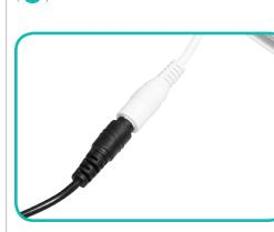
Connect the Jumper Cord to the Transformer using the barrel connectors.
