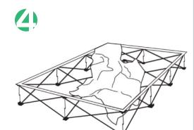
• Starting at one corner, attach loop on the graphic to hook on the frame.
